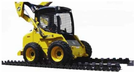
3. Slowly drive the machine over the tracks. Stop halfway over the track chain.
