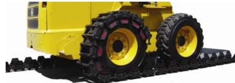
4. Fold the back end of tracks over the back tire of the machine.
