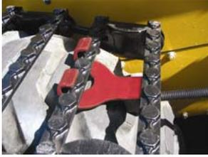
7. Insert installation tool under the first open section of the track.
