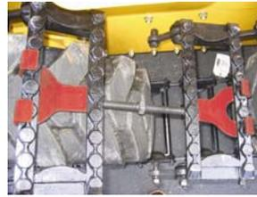
8. Connect the other end of the installation tool to the opposite section of the track.
