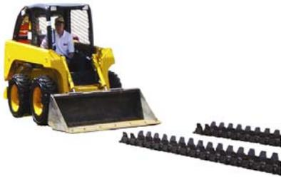
1. Make sure that both tracks are parallel to each other and of equal distance to the machine. Remove as much slack as possible.
