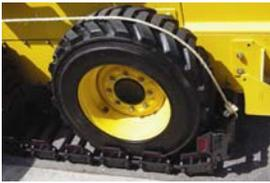
4. Drive forward enough to pull the track halfway over the rear tire.
