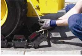
1. Tie one end of the rope to the last pad of the track chain.
