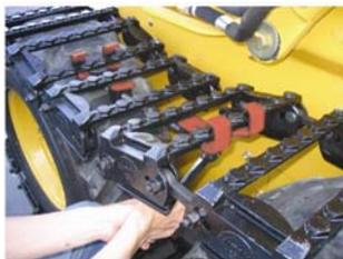
13. Once the carriage bolts are tight, loosen the installation tool.
