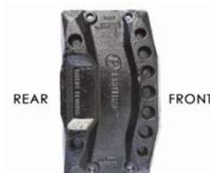
Protrac Magnum is directional. When the track is mounted on the machine, the thick solid bar should point to the front of the machine, when looking at the top of the track.
