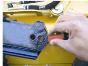
10. When the open Protrac track sections get close enough together, insert the ends of the dog-bone links into their respective slots.
