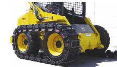
14. Remove the installation tool from the track and then move the machine forward until there is an open space to insert the carriage bolt on the inside of the track. Tighten the bolt.
