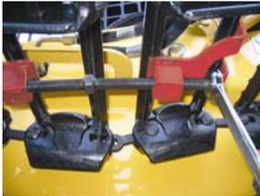
9. Put ratchet on the square end of the threaded rod. Use the ratchet to bring the two ends of the track together.
