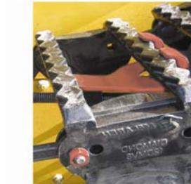
12. Tighten the carriage bolts. You can tighten to 100 pounds of torque pressure or use an automotive air gun.
